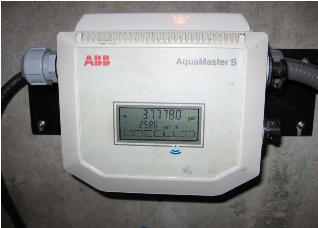
Figure 2. “AquaMaster S” data logger installed at the Alma Aquaculture Research Station. Total accumulated flow and instantaneous flow rate are displayed.
